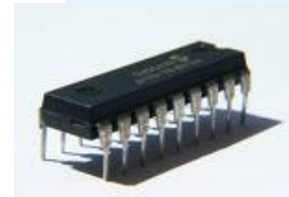
SSI: Small scale integrated circuit
