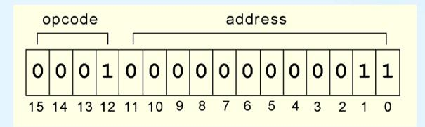
We see that the opcode is 1 and the address from which to load the data is 3.
