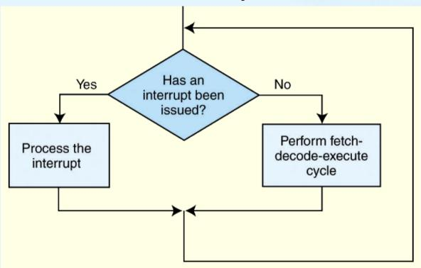
The next slide shows a flowchart of "Process the interrupt."
